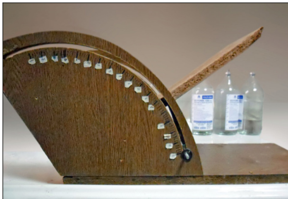
Figure 2. Inclined plane test system.
