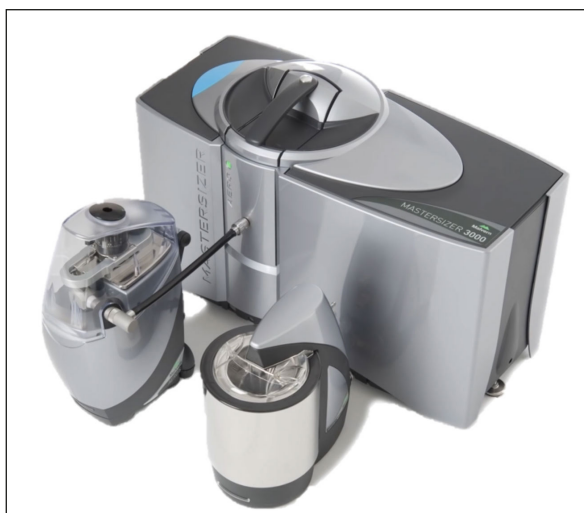
Figure 8. The Mastersizer 3000 is able to analyze the size of the granules using laser diffraction.
