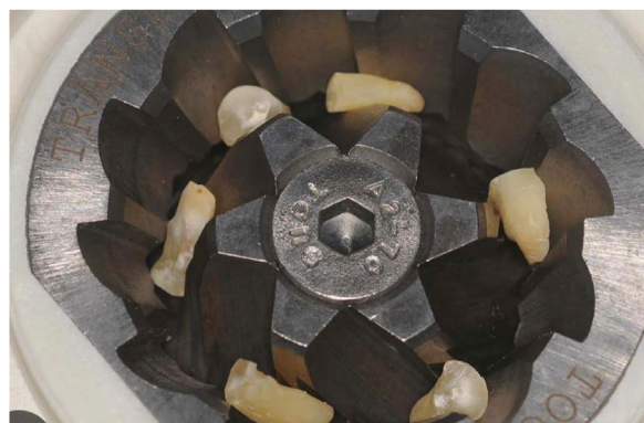
Figure 4. Tooth fragments are positioned in the Tooth Grinder® (CE).
